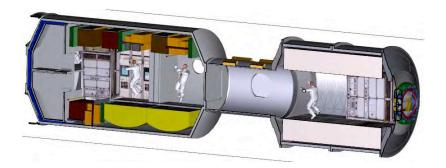
Notional Deep Space Transit Vehicle Longitudinal Arrangement, Section
